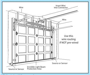
FIG. 4-6 Wire routing.
